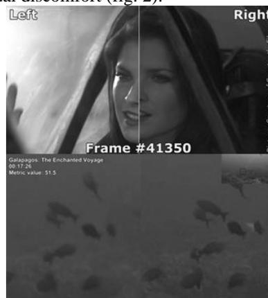
Fig. 2 Discrepancies between left and right eye images; (upper stereo pair from Resident Evil) asymmetry in luminance; (bottom stereo pair fragment from Galapagos: The Enchanted Voyage) asymmetry in sharpness;
